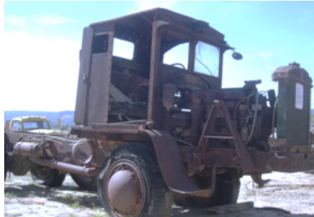
1930 Coleman showing the large dish-like hubcaps that house the front wheel drive
